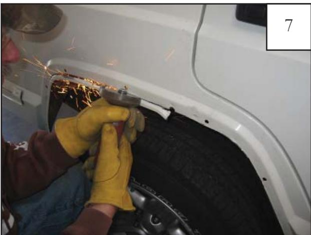
Use a cut off saw to cut the rear fender along marked line.
