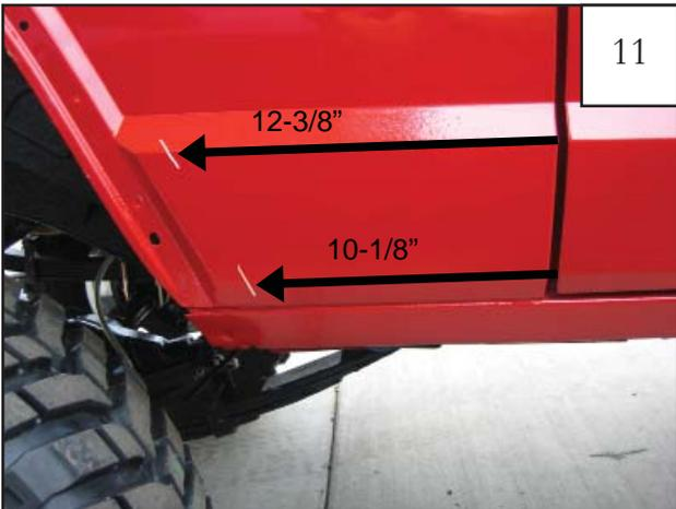
**(For 2-Door Vehicles Only)** Use a grease pencil or removable marker to make a line parallel with the wheel well opening  $12\text{-}\frac{3}{8}$ " from the door edge seam along style line and  $10\text{-}\frac{1}{8}$ " on lower style line.
